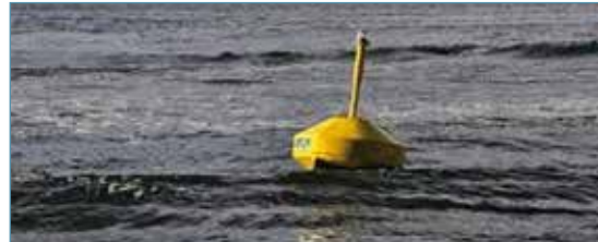
Accumulated Ocean Energy 1-12 scale device testing in Sooke Basin - Vancouver Island
