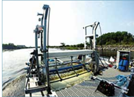
Floating ducted crossflow turbine (Mavi Innovations)
