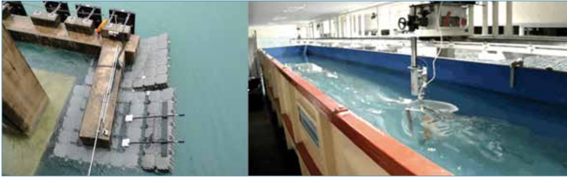
Floating hinged turbine support frame to house tidal turbines and vortex induced vibration devices. (Left) & Scaled (1:3) tidal turbine in tow tank (Right)
