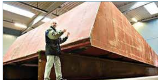
Crestwing prototype 10 meter wide 30 meter long 2,5 meter high with a weight of 60
